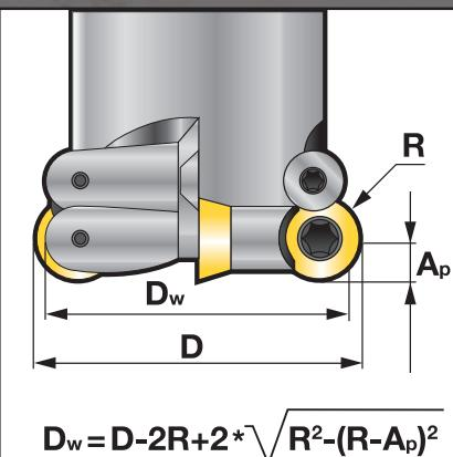
The "fz" indicated above is for an overhang of  $3xD$ . The values are calculated based on the recommended thickness of the chip "hm".
